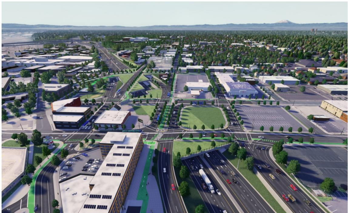
The highway cover would connect both sides of I-5, reducing the physical barrier of I-5 between neighborhoods to the east and west of the highway while providing additional surface area above I-5. The added surface space would provide an opportunity for new and modern bicycle and pedestrian facilities and public spaces when construction is complete, making the area more connected, walkable, and bike friendly.
